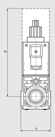
d = Space required for replacing solenoid
