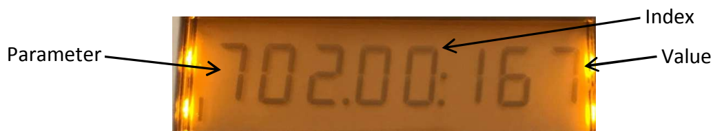
Figure 7-1: LME7 Fault History Example with Indexes
